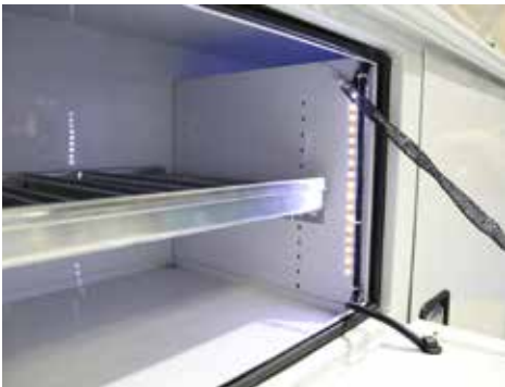
LED COMPARTMENT LIGHTS
